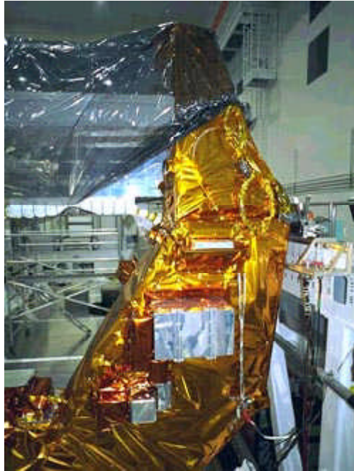
HOST payload with SAMS-FF ready for integration on the space shuttle for STS-95. The SAMS-FF control and data acquisition unit can be seen in the lower left corner.
