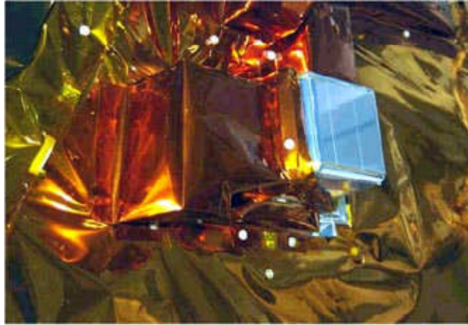
SAMS-FF control and data acquisition unit mounted on the HOST payload.
