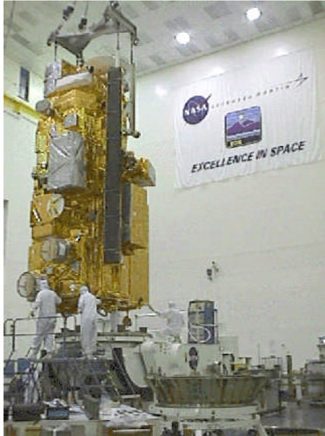
EOS spacecraft following shock separation testing at Lockheed Martin Missiles & Space, Valley Forge, Pennsylvania.
