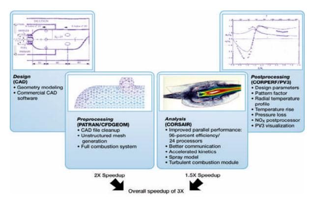
Typical results for the National Combustion Code (NCC), a combustor design and analysis system.
