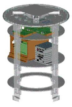
Preliminary layout of the Direct Data Distribution experiment in a NASA Goddard Space Flight Center Hitchhiker-G canister.
