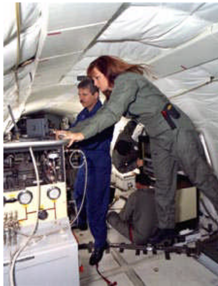
Cool flame experiment aboard NASA's KC-135 reduced-gravity aircraft.
