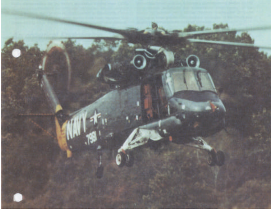
Figure 5: Navy/Kaman Aerospace XH-2D/CCR flight test demonstrator with circulation control rotor (CCR).
