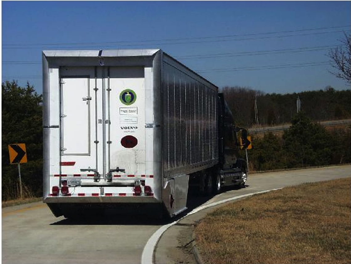
Figure 8 Pneumatic heavy vehicle (PHV) with TE blowing
