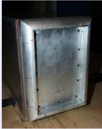
4 Blown Slots & Jet Turning on Rear Doors of Wind-Tunnel Model
