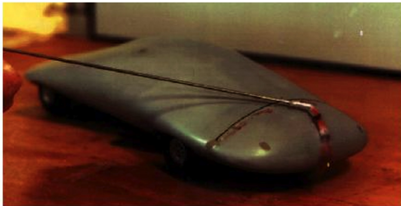
Figure 5 Futuristic Car with Aft CC (Sliding Block Adjustment)
