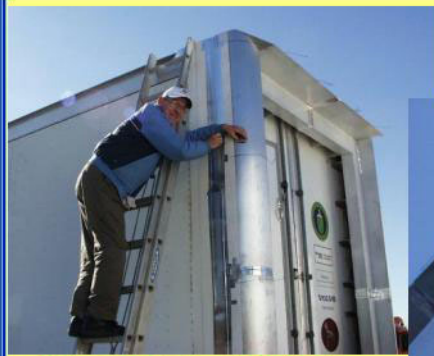
Setting Slot Heights and Confirming Jet Turning at Low Blowing Rate on Aft Door of Trailer
