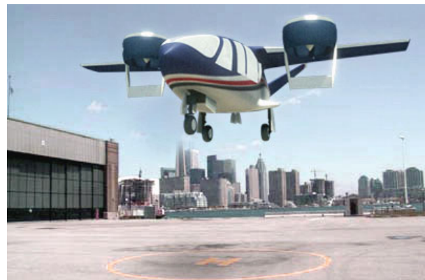
Figure 6: Far-term 15-year advanced Tilt Nacelle Vertical Takeoff and Landing (VTOL) concept that utilizes a Multi-Gas Generator Fan propulsion system to reduce engine-out sizing penalties, and a Circulation Control Nacelle to externally expand the ducted propeller flow pneumatically to reduce the ground plane velocities and permit matching of the cruise and hover disloadings. This mission is envisioned as a Air-Taxi that accomplishes very high utilization to
