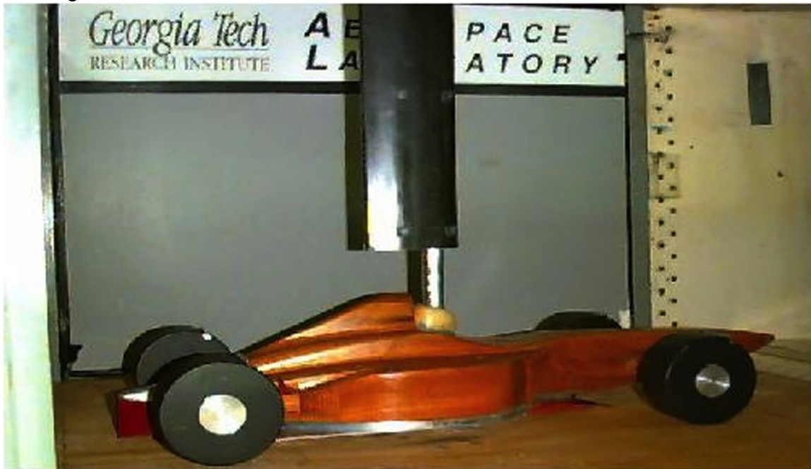
Figure 2 Formula 1 car with CC blowing on bottom plate
