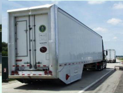
Rear View of Test and Control Vehicles, Showing Blown Tufts Turning
