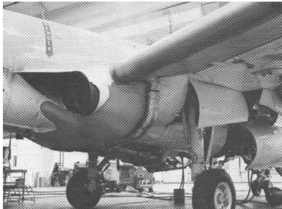
Navy Grumman A-6A Intruder All Weather Bomber, modified to demonstrate Circulation Control High Lift Wing Concept flew in 1979.
