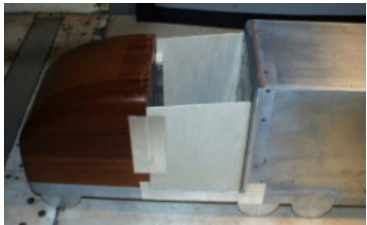
Figure 10 – Side Plates and Trailer Top Blowing: a Practical Solution to the Cab Gap Problem
