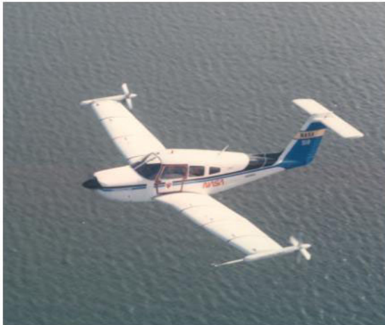
Wingtip Turbine Wake Vortex Experiment, Paterson et al, 1988, NASA Langley
