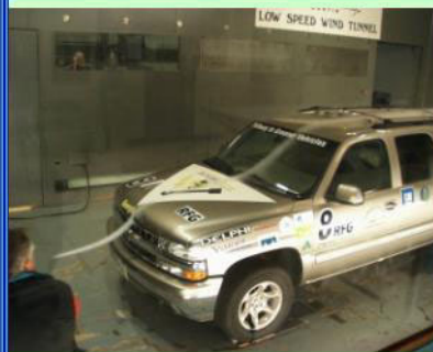
Smoke Flow over Unblown SUV, Testing in Lockheed 16' x 23' Low Speed Wind Tunnel, Marietta GA
