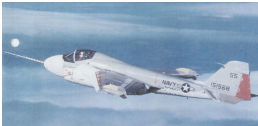
Figure 4: Navy/Grumman A-6A/CCW flight test demonstrator with circulation control wings (CCW).
