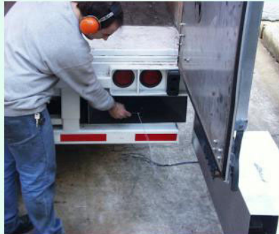
Tuft Showing Flow Uniformity at Diffuser Center
