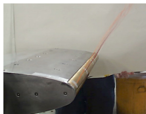
single slot blowing (lower) 180 deg redirection of the wall jet
