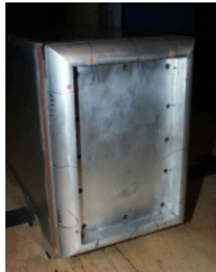
Figure 7 - Drag Reduction or Augmentation on Blown Trailer with 90° Turning Surfaces, plus Flow Visualization of Jet Turning
