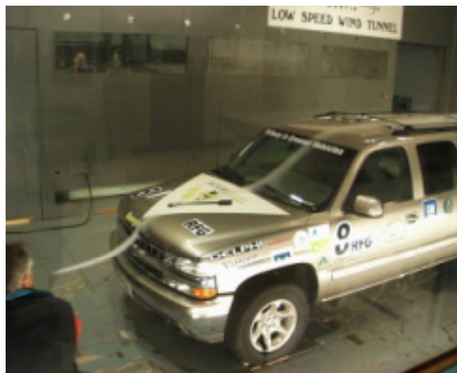
Figure 24- GM Suburban Test Vehicle Undergoing Smoke Flow Visualization in the Lockheed 16' x 23' Wind Tunnel Test Section
