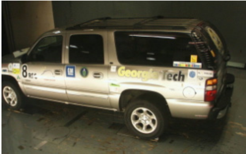
Figure 25- GM Suburban Test Vehicle Undergoing Tuft Flow Visualization in the Lockheed Wind Tunnel
