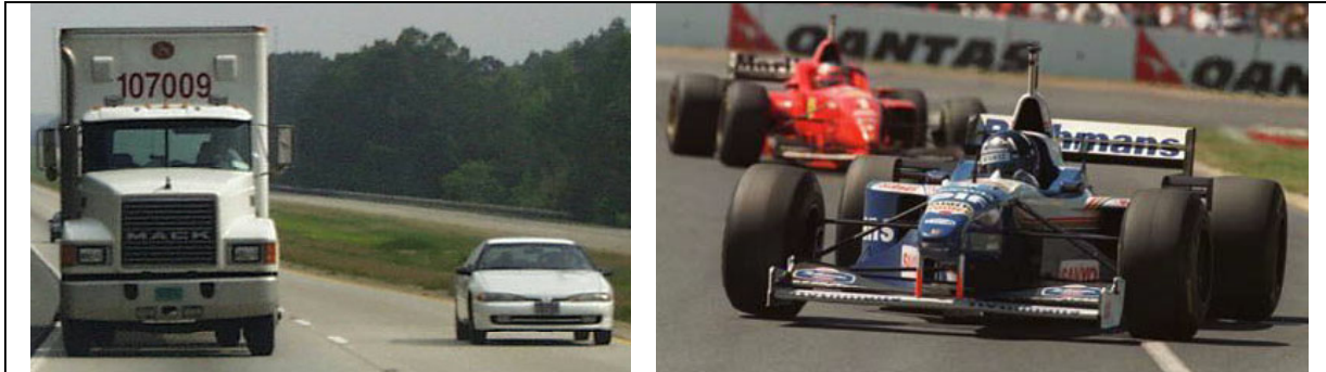
Figure 3 Large Heavy Vehicle and passenger car: radiator presents large frontal area to flow, thus significant drag. F1 & Indy cars: pods or ram scoops are necessary evils - speed draining drag sources
