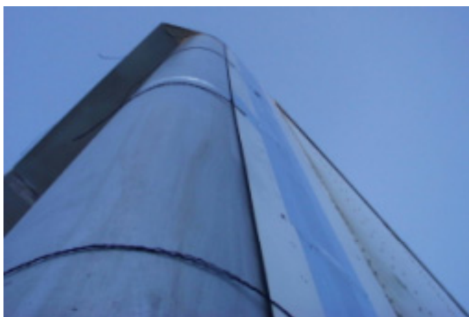
Figure 13 Right Rear Corner View, Looking Up, with Tufts Showing 90° Jet Turning
