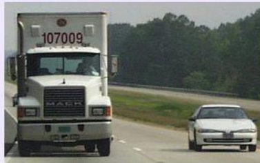
Heavy Vehicle vs Conventional Car ~Much Larger Frontal Area and Drag
