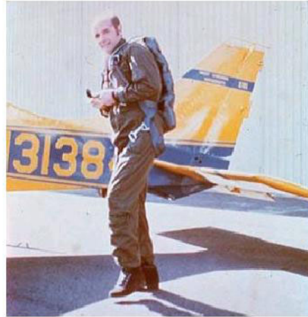
Note spin chute below tail and parachute on his back
