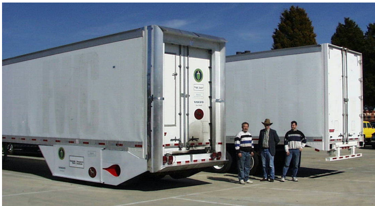
Figure 12- PHV Pneumatic Trailer (left) and Baseline Reference Unmodified Trailer (right)
