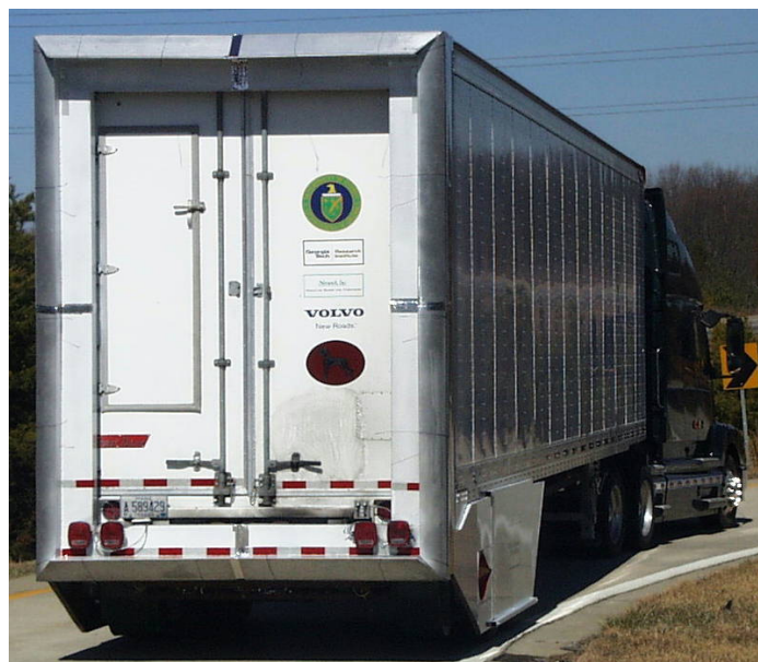
Figure 15- On-road PHV Test Vehicle Rear View with Jets Blowing and Tufts Turning
