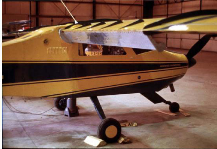
Flap in process of retracting, by folding forward into cavity 17
