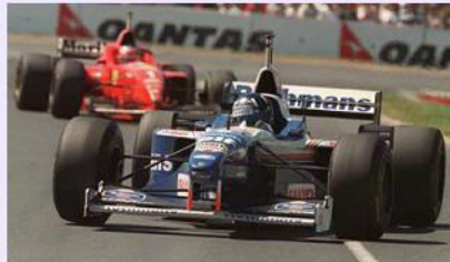
Large Frontal Area and Drag due to Radiator Pods on Formula 1 or Indy Racer
