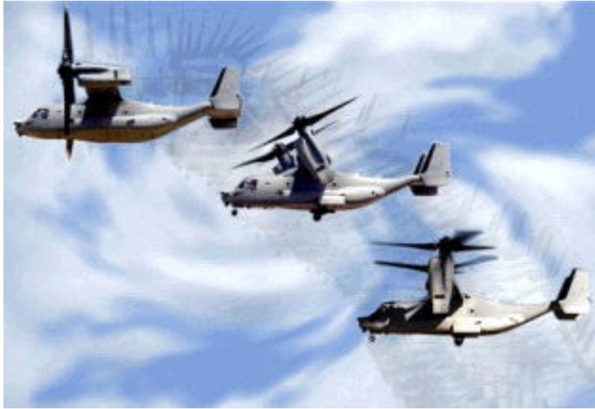
Figure 1: Bell Boeing V-22 Osprey transitioning from helicopter to aircraft mode (Photo courtesy US Navy).
