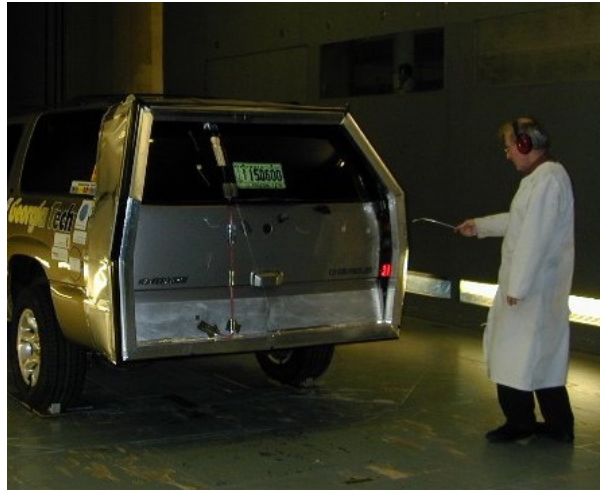
Figure 27- Modified PSUV Blown Test Vehicle in the Lockheed Low Speed Wind Tunnel
