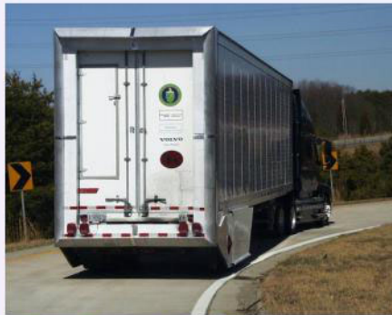
Rear View with Jets Blowing
