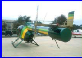
Circulation Control Tail Boom on NOTAR
