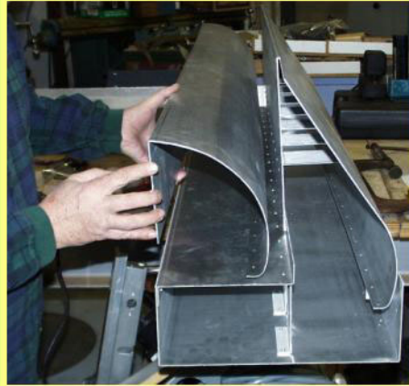
Plenums, Slots and Turning Surfaces, Showing 90° (left) & 30°
