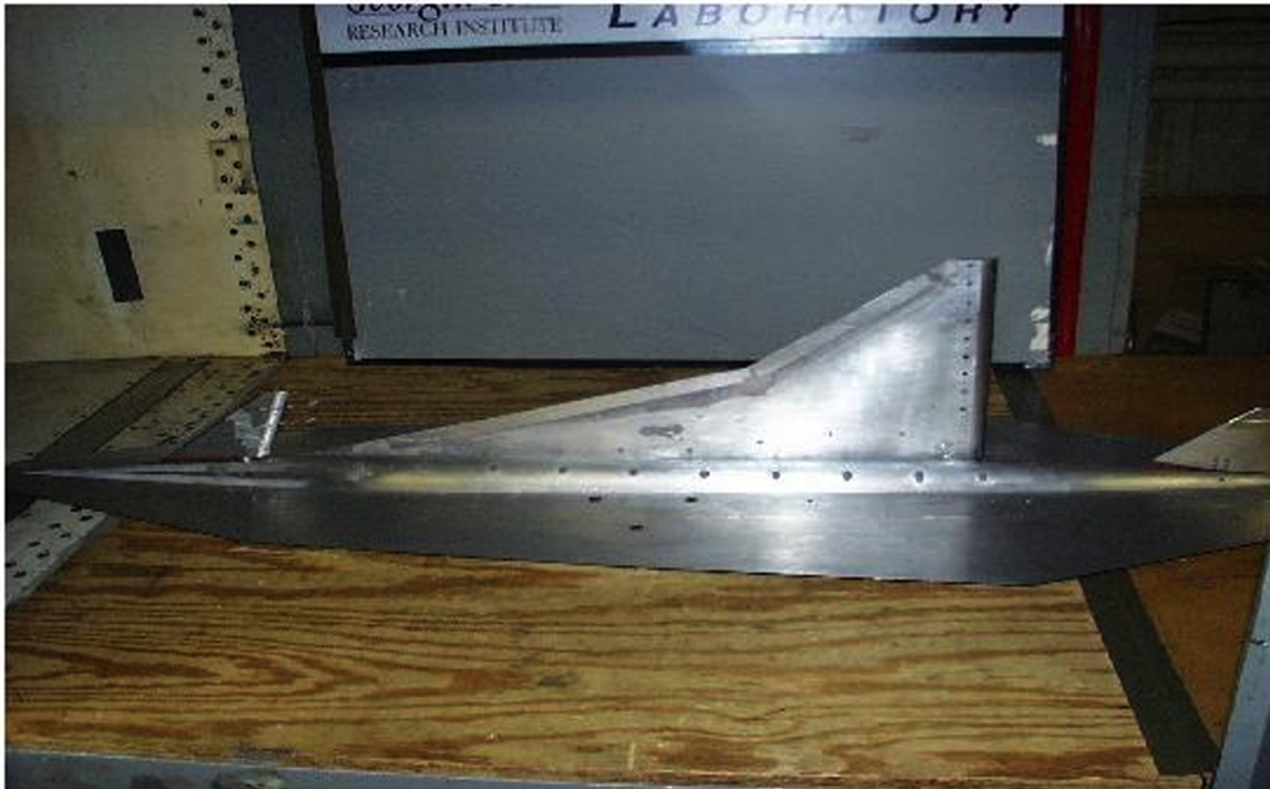
Figure 6 High-speed civil transport with CC blowing on canard TE, Wing TE, and Wing LE
