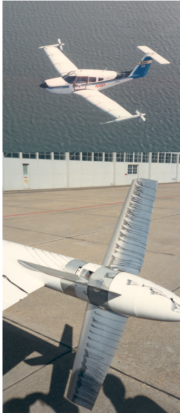
Figure 12: Piper Arrow GA aircraft modified with a wingtip turbine system in 1988 to investigate the potential for extracting power during cruise for replacement or elimination of APUs and improved cruise efficiency.
