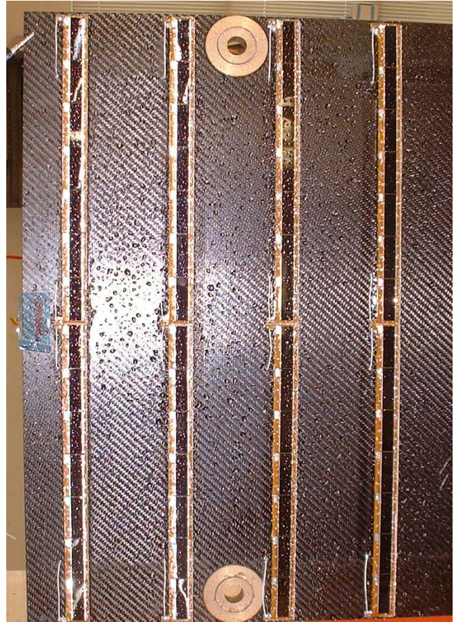
Figure 9 – Photovoltaic Receivers Undergoing 500 V Wet Hi-Pot Testing
