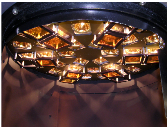
Figure 8) Photograph showing the 12 filtered lamps of the 36 lamp IR source.
