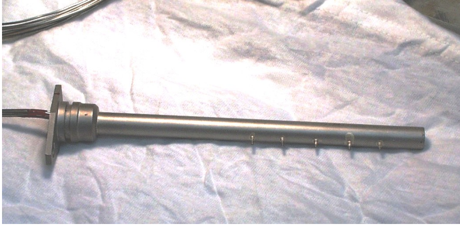
Figure 6.—Photograph of thermocouple rake used in these tests.
