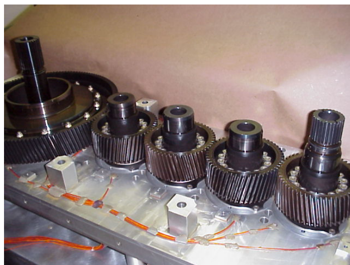
Figure 8.—NASA High-Speed Helical Gear Train Test Facility components.
