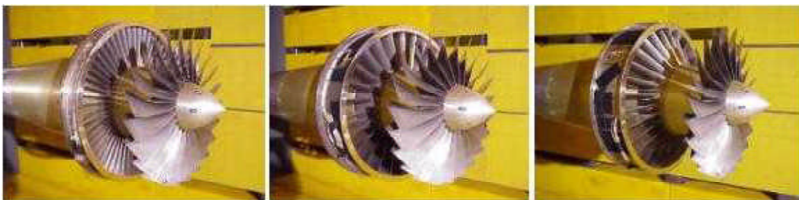
Partially assembled fan stages showing the three outlet guide vanes (OGV) tested. From left to right, the baseline 54-vane radial OGV, and the 26-vane radial OGV and the 26-vane swept OGV.
