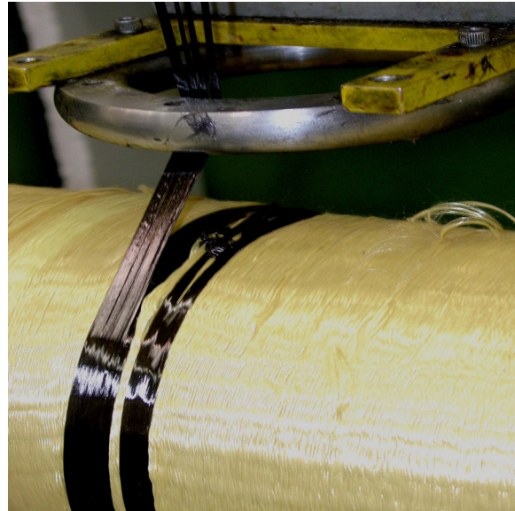
Figure 7 Covering the braid with epoxy coated carbon fiber
