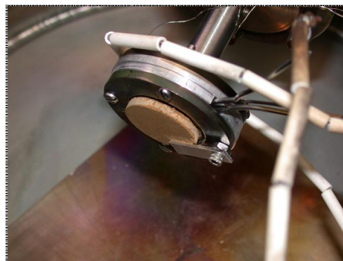
Figure 3: Soil sample mounted on an electrically heated target holder
