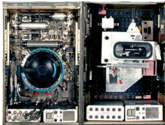
Engineering models of the Fluids and Combustion Facility. The Combustion Integrated Rack (CIR) is shown on the left; the Fluids Integrated Rack is shown on the right.
