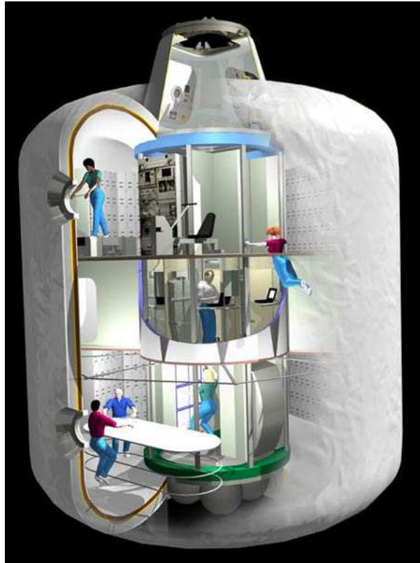
Figure 3.11.: The proposed design for the Transhab, that was originally designed to be part of the International Space Station. It is comprised of three main sections that provide different capabilities to the crew. Courtesy of NASA.
