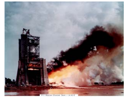
S-1C-T Five F-1 Engine Hot Fire Cluster Test at Marshall Space Flight Center (MSFC) - 1965
