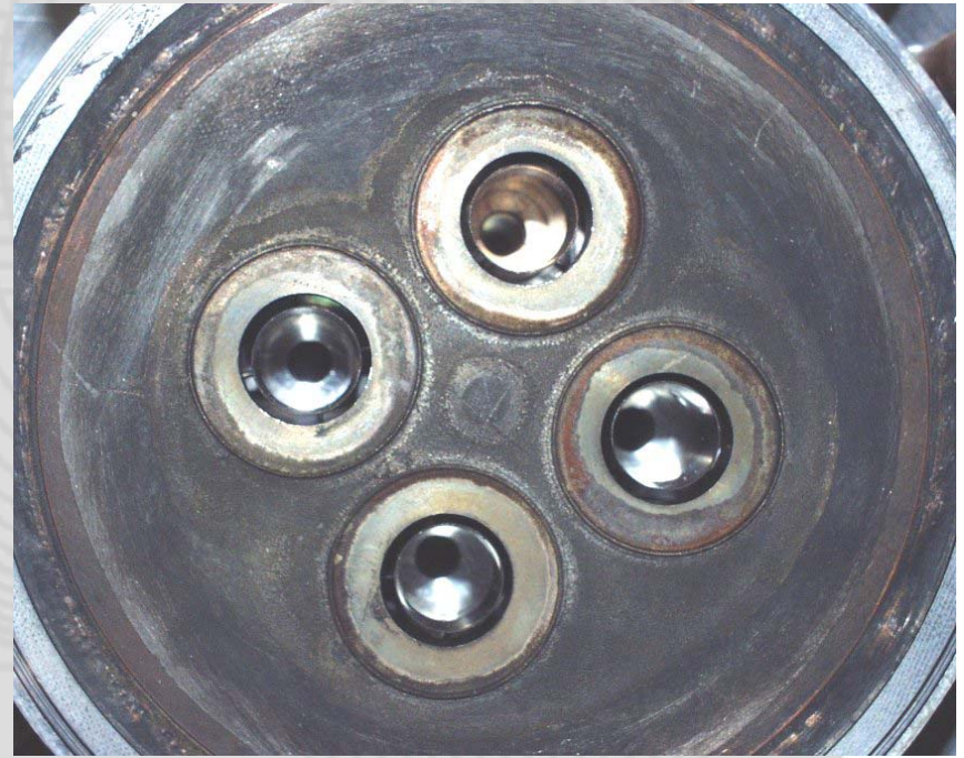
Faceplate with large gasdynamical elements after 3 tests and 100 s run-time
