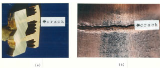
Fig. 11 Photos of cracked nozzle throat section of a water cooled thrust chamber
