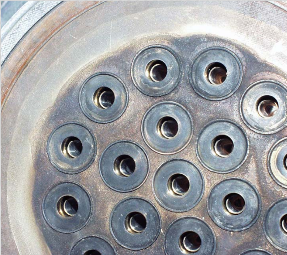
Faceplate after 3 tests and 115 s run-time
