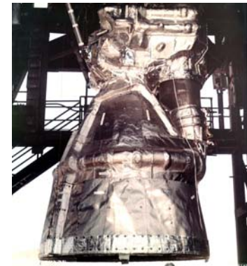
Thermal Protection System (TPS) Installed on Single F-1 engine - 1965
