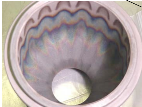
R512 Disilicide-Coated C103 Chamber Replaced by Pt-Ir Alloy Chamber
