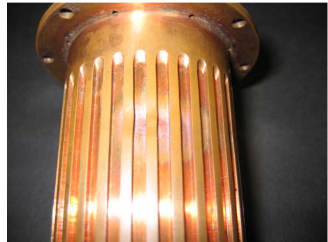
Discoloration and deformation at 90 cycles ( 1.5'' \times 0.6'' )
