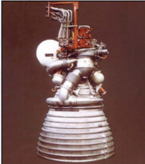
J-2 Saturn V S-II & S-IVB Stage Engines Saturn IB S-IVB Stage Engine
