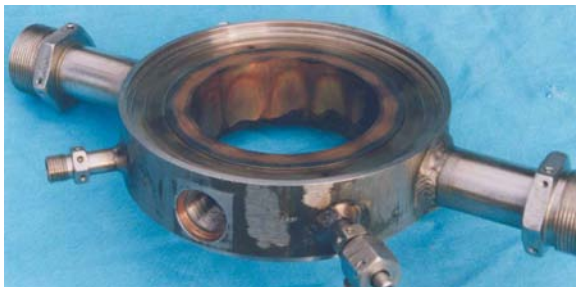
Figure 18: Chamber wall section after 12 tests and 450 s run time
