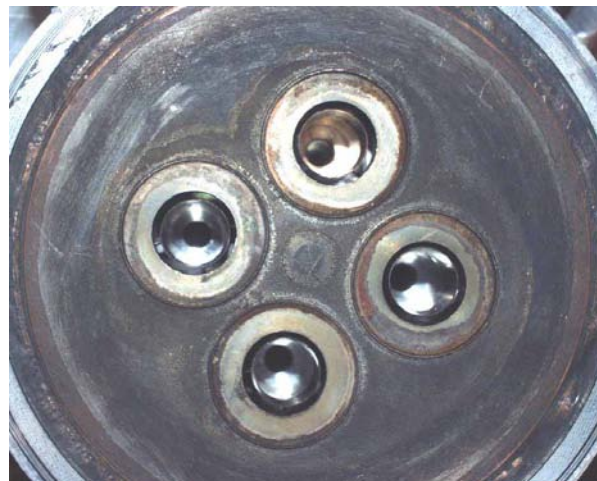
Figure 15: Injection head with large gasdynamic coax elements after 3 tests
