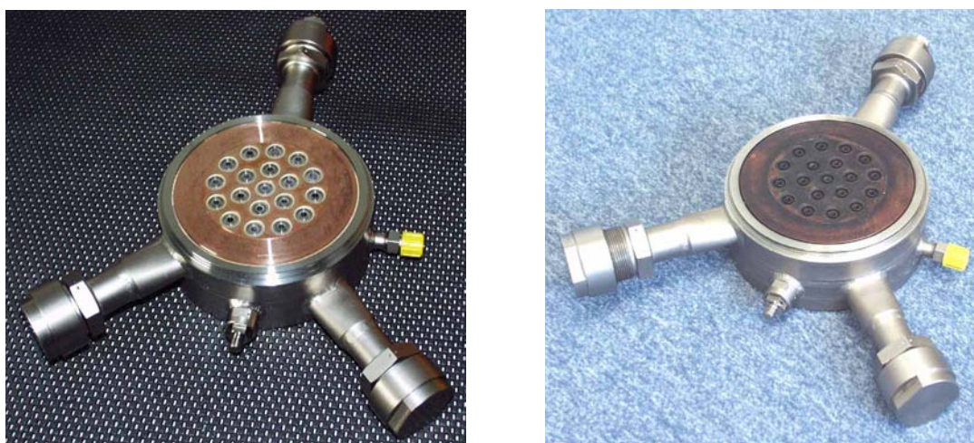
Figure 20: LOX-kerosene injector head before and after 3 tests and 110 s run-time showing soot deposition
