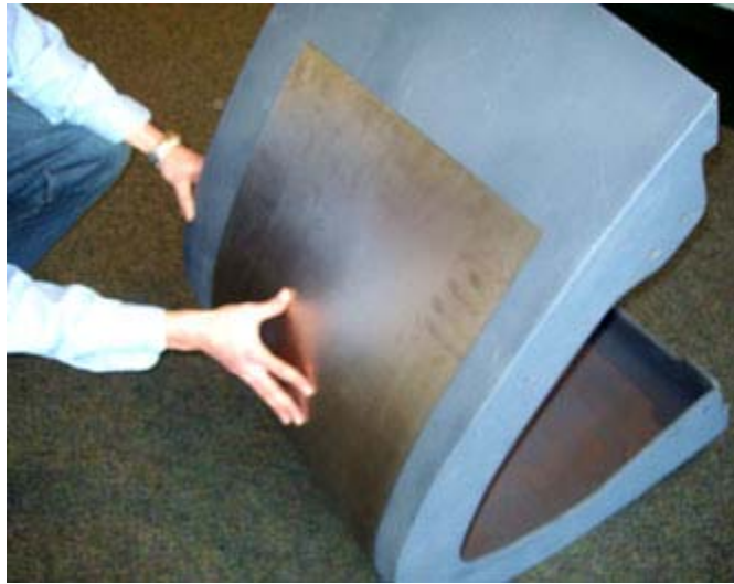
Representation of concept for a refractory metal overwrap. Mockup of the space shuttle orbiter RCC panel 9.
