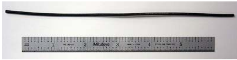
Piece of \text{Ni}_{30}\text{Pt}_{20}\text{Ti}_{50} 0.056-in.-diameter wire processed by high-temperature swaging.
