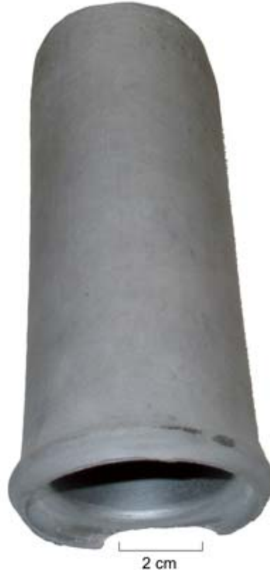
NNS forming of a rhenium heater head.
