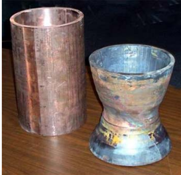
A comparison of a welded cylinder and a liner preform after completion of metal spinning. The cylinder is 18 in. tall.
