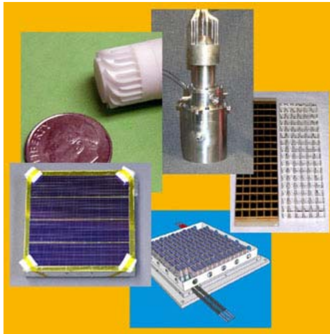
Collage of hardware and designs developed during the RPCT phase-I development contracts, representing Brayton, Stirling, thermoelectric, and thermophotovoltaic technology.
