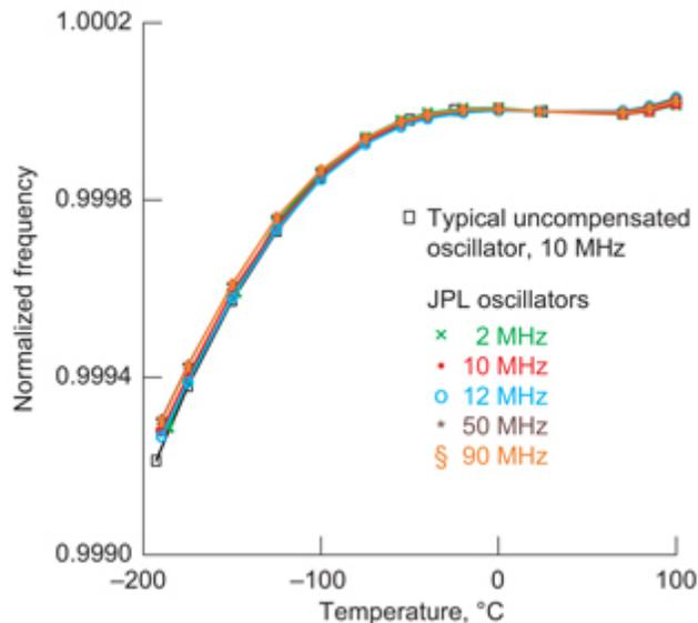
*Normalized output frequency of six oscillators versus temperature. Frequency normalized*
