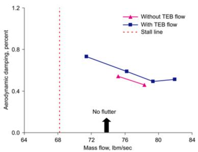
Aerodynamic damping for the trailing edge blowing (TEB) fan calculated with the TURBO-AE aeroelastic analysis code.
