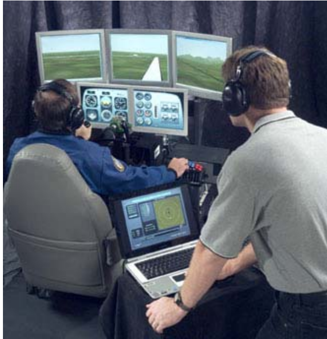
Pilot performing an approach to landing using the Ice Contamination Effects Flight Training Device, with instructor observing pilot reactions.
