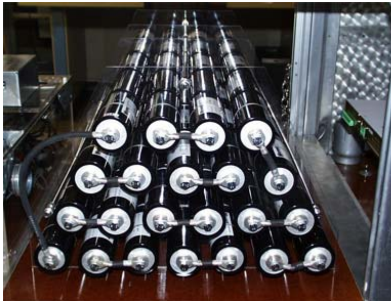
The Hybrid Power Management (HPM) Program applied to the Next Generation Launch Transportation (NGLT) Project. Top: Fuel cell laboratory with PEM fuel cells and a bank of ultracapacitors. Bottom: Bank of 110 ultracapacitors connected in a series configuration.
