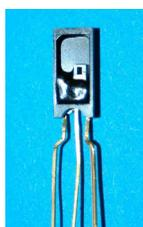
(b) Capacitance type humidity sensor.
