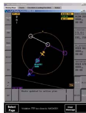
Figure 16. Maryland Mid-Atlantic SATSLab ‘Cockpit Associate’ aids the pilot in flying safely and proficiently by conducting situation assessments, and providing recommendations and advisories.
