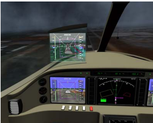
Figure 7. Advanced cockpit concept utilizing a PFD with HITS flightpath guidance, a MFD with navigational tools, and HUD for out-the-window monitoring for improved flightpath accuracy and situation awareness in IMC.
