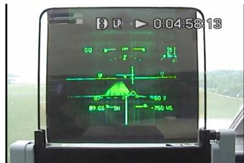
Figure 12. Maryland Mid-Atlantic SATSLab HUD with EVS allows for increased safety and performance on approach to landing.
