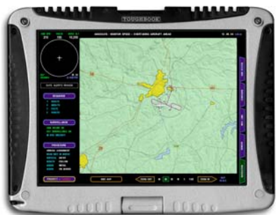
Figure 15. Virginia SATSLab Electronic Flight Bag provides the pilot navigational information and HVO functionality to allow for increased situation awareness and performance.
