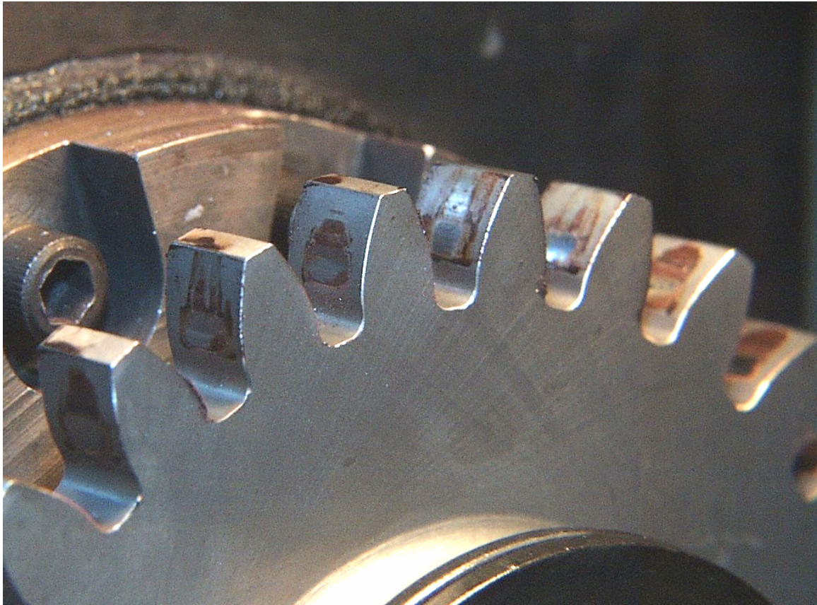
Figure 11.—Condition of the driven gear after 1 hr of testing for test number 7 having test conditions of no lubricant, 705 rpm shaft speed, 2 ft-lb torque, and ambient air atmosphere.
