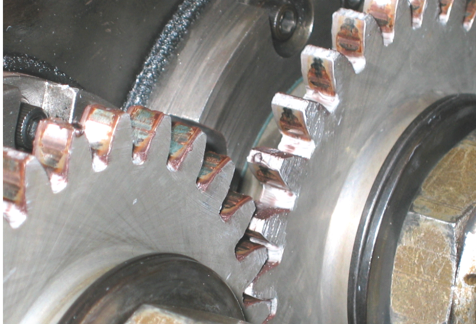
Figure 2.—Condition of the test gears after 3 hr of operation for test number 1 having test conditions of perfluoro type grease, 515 rpm shaft speed, 5 ft-lb torque, and ambient air atmosphere.
