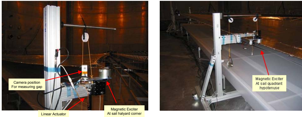
Figure 4. Magnetic Exciter System Configuration
