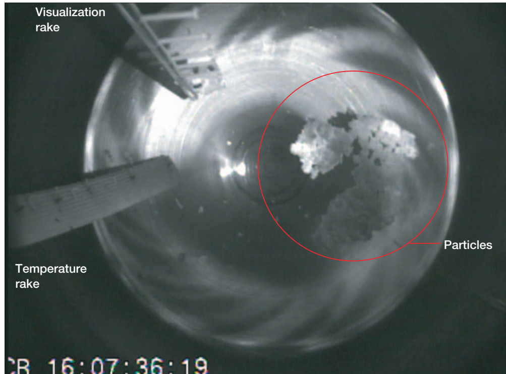
Figure 6.—Image of solid hydrogen image (enclosed in circle), 2001. Full mass on helium surface, 0.3159-m-diameter Dewar.
