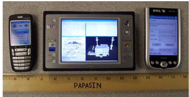
Figure 3. Responder IEPs. From left to right are the Smartphone, tablet, and PDA. All are running the SSRL Responder Tool. Ruler units are inches.
