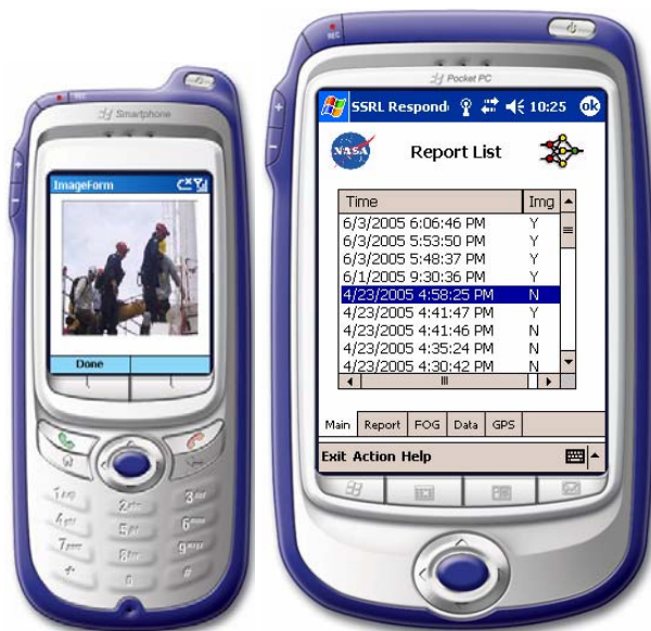
Figure 6. Part of the report user interface on the Smartphone and PDA responder IEPs. On the Smartphone, the user has selected the image associated with a report (created during one of the field tests) and is viewing it. On the PDA, the user is viewing the chronological list of reports.
