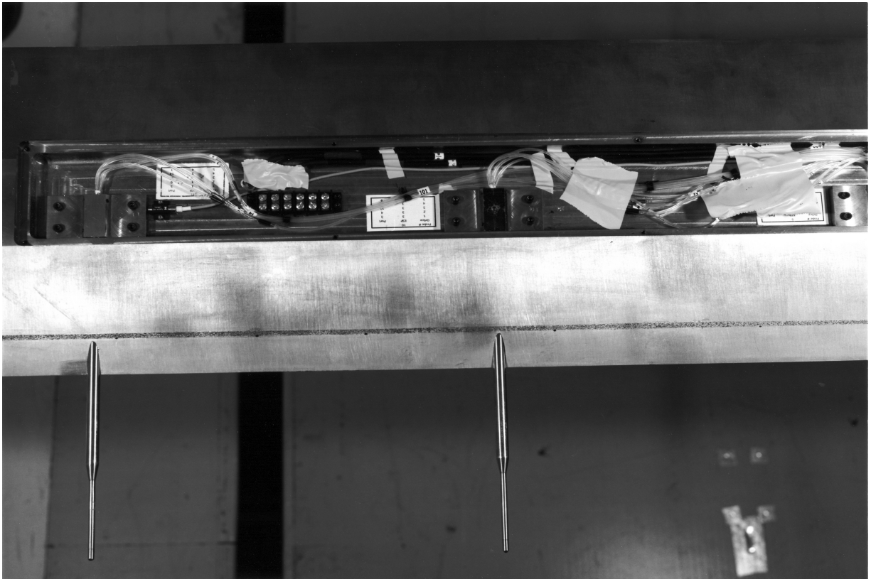
Figure 5. Survey rake with instrumentation hatch removed.
