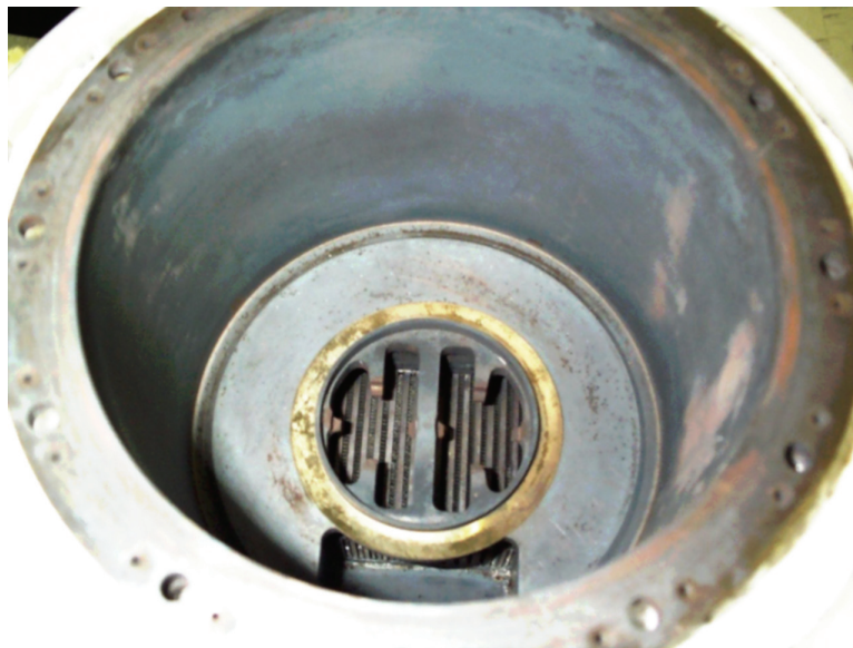
Figure 8. RLSE test stand TCO with catalyst bed removed.
