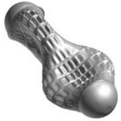
6. Mode number 13, Frequency 199.4 Hz Shape: i=2, j=2 circumferential-axial mode (1 of 2)
