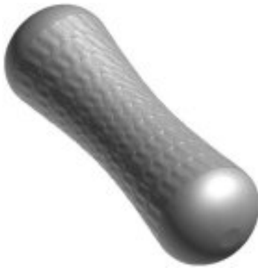
4. Mode number 6, Frequency 150.6 Hz Shape: First torsion
