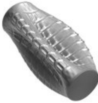
2. Mode number 4, Frequency 143.2 Hz, Shape: i=3, j=1 circumferential-axial mode (1 of 2)
