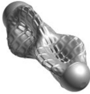
5. Mode number 15, Frequency 177.6 Hz Shape: i=3, j=2 circumferential-axial mode (1 of 2)
