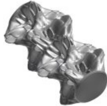
15. Mode number 28, Frequency 322.3 Hz, Shape: i=4, j=4 circumferential-axial mode (1 of 2)
