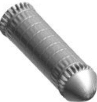
8. Endcap mode 2, Frequency 217.5 Hz
