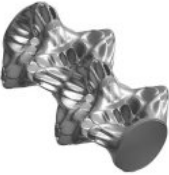
13. Mode number 20, Frequency 312.3 Hz, Shape: i=3, j=4 circumferential-axial mode (1 of 2)
