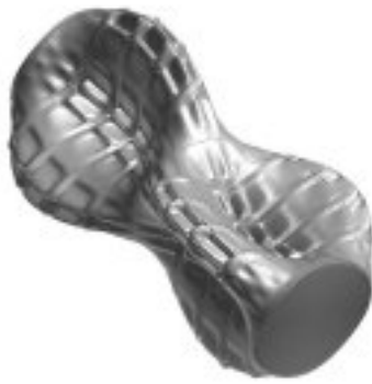
4. Mode number 8, Frequency 175.4 Hz, Shape: i=3, j=2 circumferential-axial mode (1 of 2)
