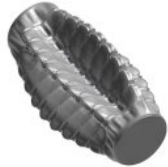
42. Mode number 72, Frequency 386.5 Hz, Shape: i=5, j=1 circumferential-axial mode (1 of 2)
