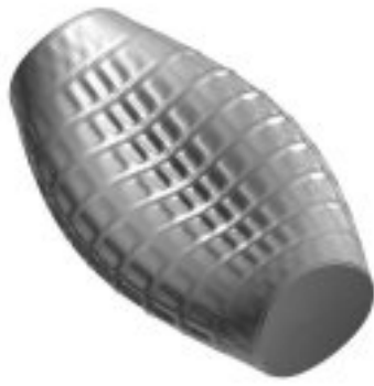
1. Mode number 1, Frequency 80.4 Hz, Shape: i=2, j=1 circumferential-axial mode (1 of 2)
