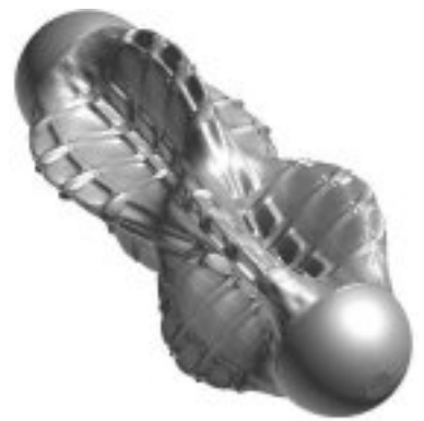
9. Mode number 29, Frequency 268.2 Hz Shape: i=4, j=2 circumferential-axial mode (1 of 2)
