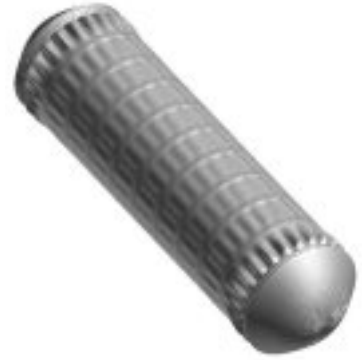
3. Endcap mode 1, Frequency 156.9 Hz
