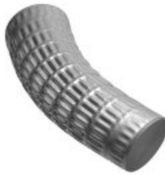
5. Mode number 6, Frequency 176.2 Hz, Shape: First bending (1 of 2)
