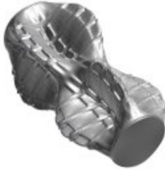
11. Mode number 18, Frequency 267.6 Hz, Shape: i=4, j=2 circumferential-axial mode (1 of 2)
