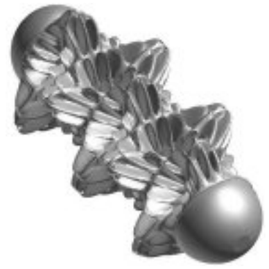
18. Mode number 73, Frequency 380.3 Hz Shape: i=3, j=5 circumferential-axial mode (1 of 2)
