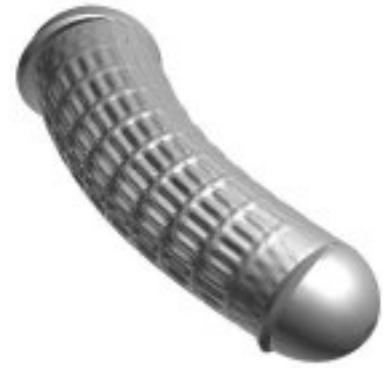
3. Mode number 4, Frequency 146.8 Hz Shape: First x-bending
