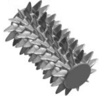
30. Mode number 52, Frequency 371.2 Hz, Shape: First panel mode on i=1, j=5 global
