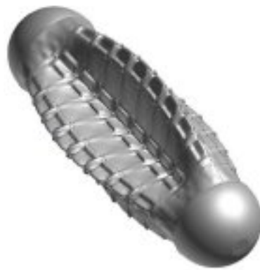
8. Mode number 25, Frequency 258.9 Hz Shape: i=4, j=1 circumferential-axial mode (1 of 2)
