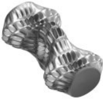
16. Mode number 26, Frequency 323.2 Hz, Shape: i=2, j=3 circumferential-axial mode (1 of 2)
