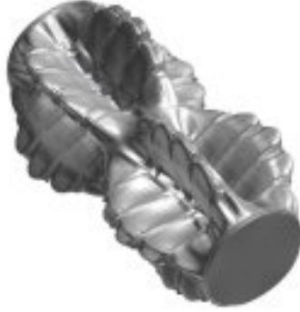
47. Mode number 82, Frequency 390.0 Hz Shape: i=5, j=2 circumferential-axial mode (1 of 2)
