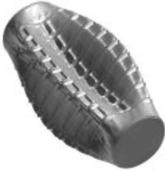
10. Mode number 16, Frequency 258.7 Hz, Shape: i=4, j=1 circumferential-axial mode (1 of 2)
