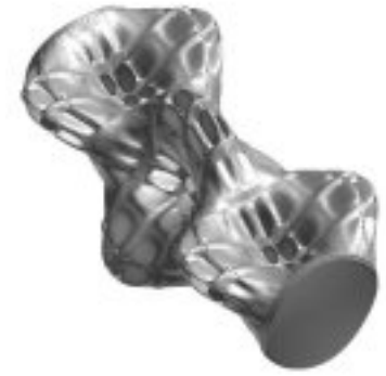
9. Mode number 14, Frequency 238.7 Hz, Shape: i=3, j=3 circumferential-axial mode (1 of 2)
