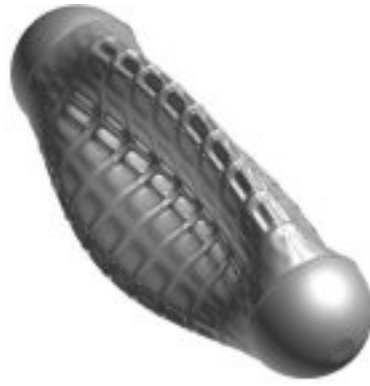
2. Mode number 7, Frequency 144.2 Hz Shape: i=3, j=1 circumferential-axial mode (1 of 2)
