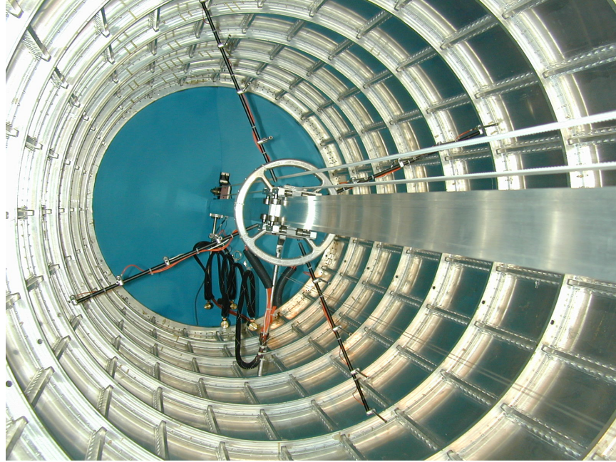
Figure 31. Interior view of ATC showing 16-microphone array mounted on traverse mechanism.
