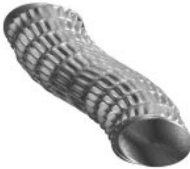
14. Mode number 24, Frequency 321.6 Hz, Shape: Second bending (1 of 2)
