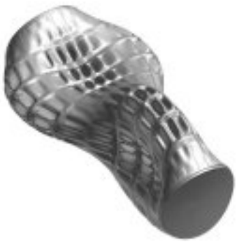
7. Mode number 11, Frequency 195.4 Hz, Shape: i=2, j=2 circumferential-axial mode (1 of 2)
