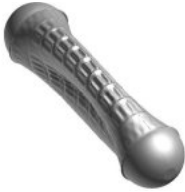
1. Mode number 1, Frequency 86.6 Hz Shape: i=2, j=1 circumferential-axial mode (1 of 2)
