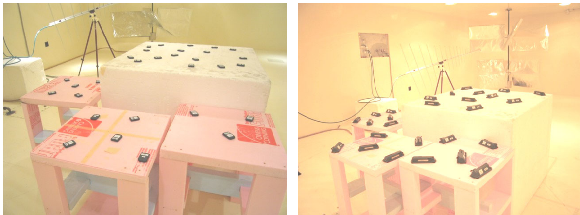
Figure 3.2-7: Test set-ups for tags in beacon mode.
