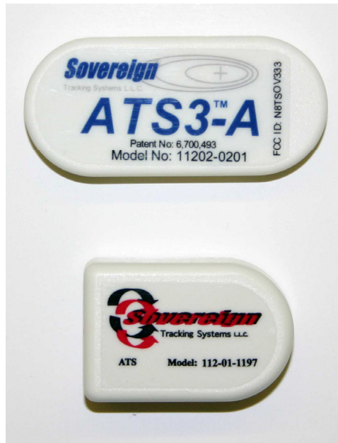
Figure 3.1-4: Sovereign ATS3-A and ATS tags (set to operate at 433.72 MHz and 417.8 MHz, respectively)
