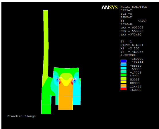
Figure 8. Local stresses in standard flange (no joint opening indication)
