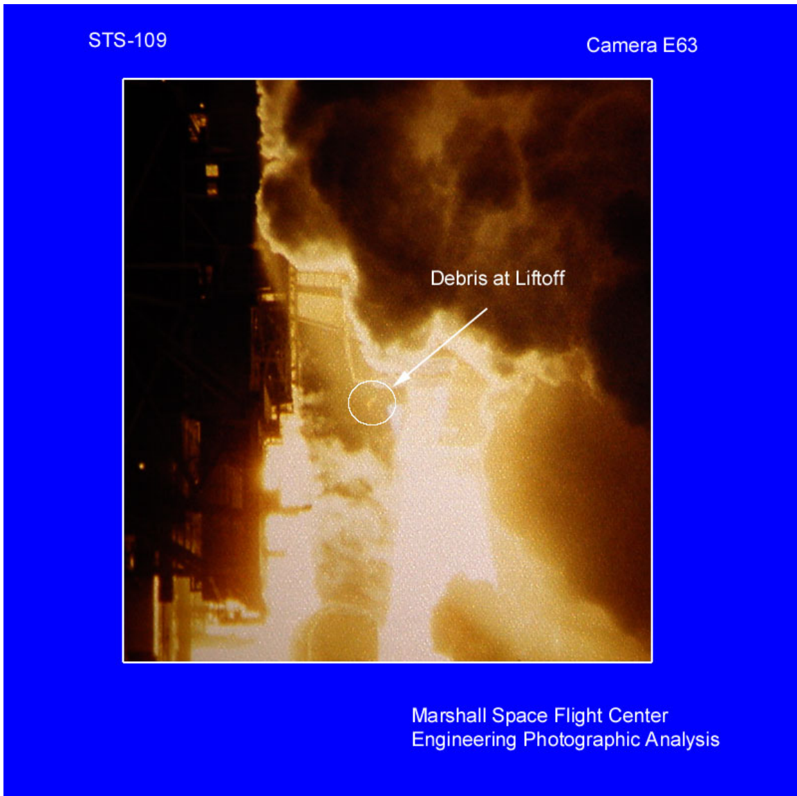
Figure 11. Film Camera E63: Debris Falling Aft
