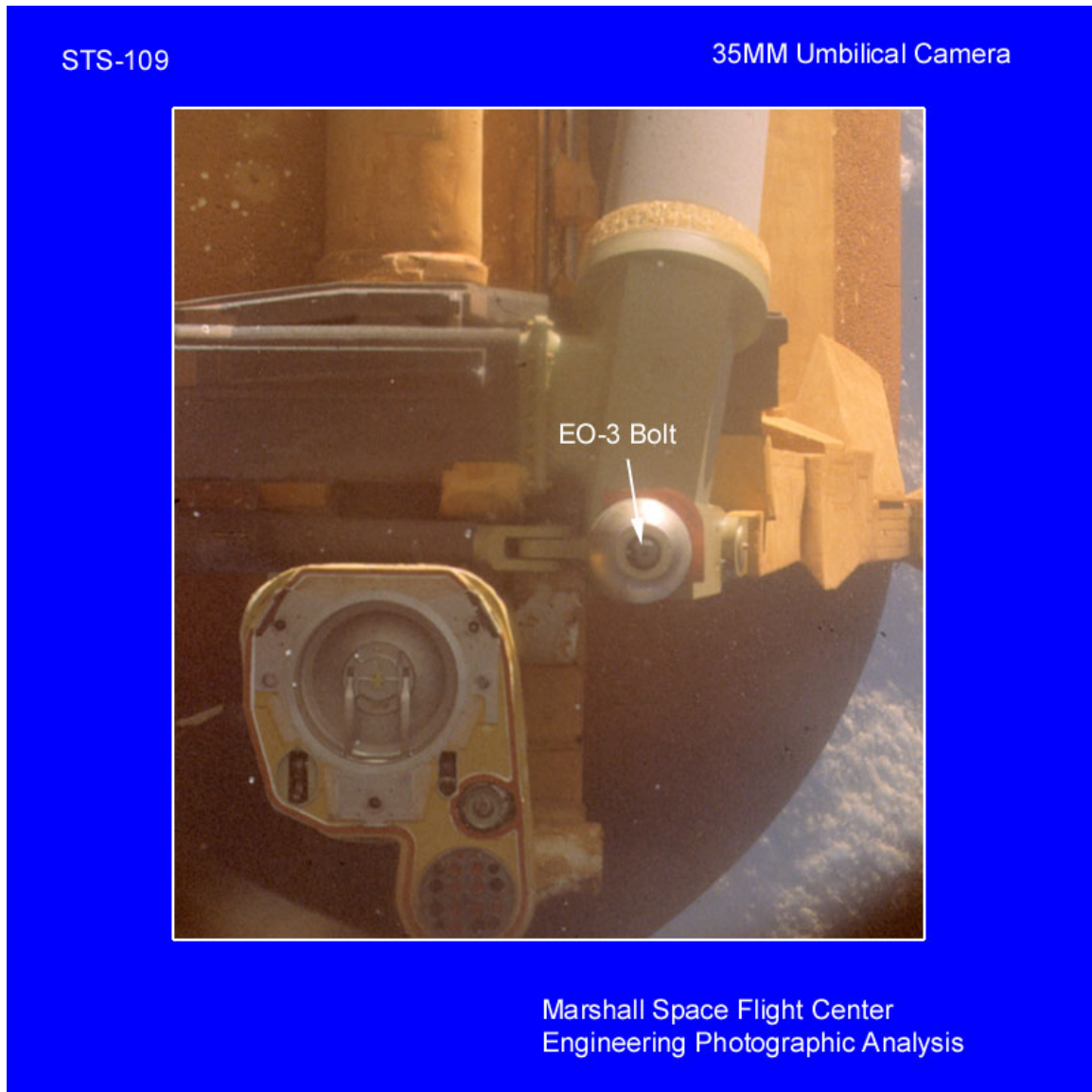
Figure 24. 35mm Umbilical Well Camera: EO-3 Bolt Protrusion
