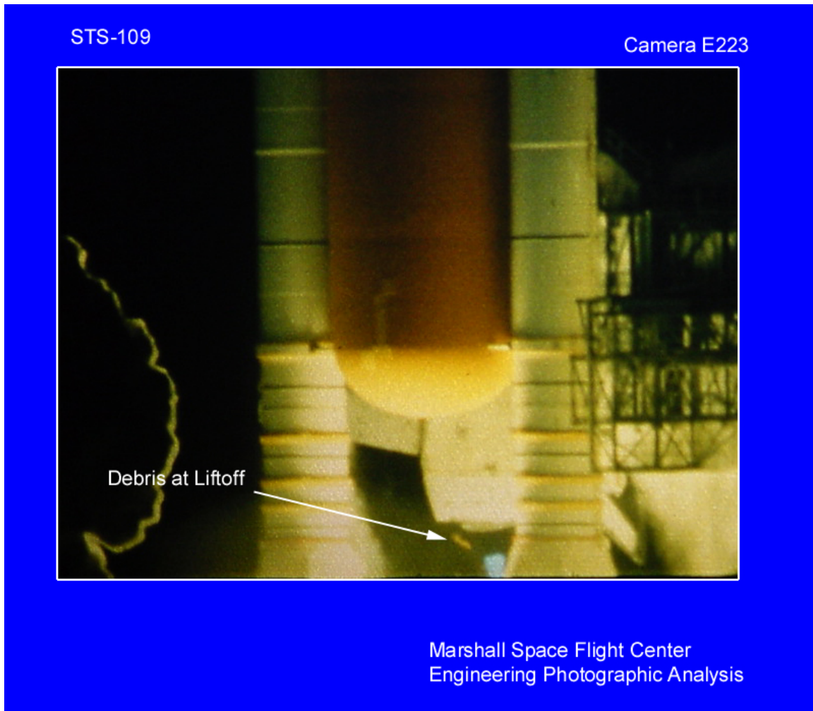
Figure 12. Film Camera E223: Debris Falling Aft
