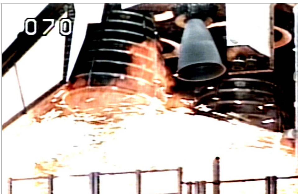
Figure 2.3.3 (A) Orange Vapor Seen Above SSME Rims Prior to Liftoff (Camera OTV070)
