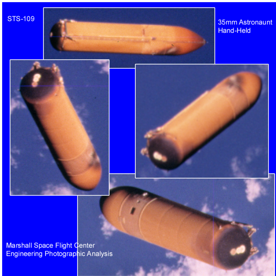
Figure 25. 35mm Astronaut Handheld Camera: ET After Separation
