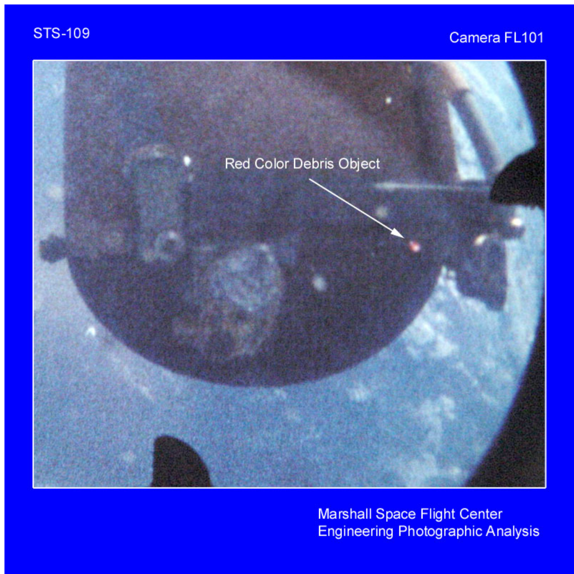
Figure 20. Film Camera FL101: Debris at ET Separation
