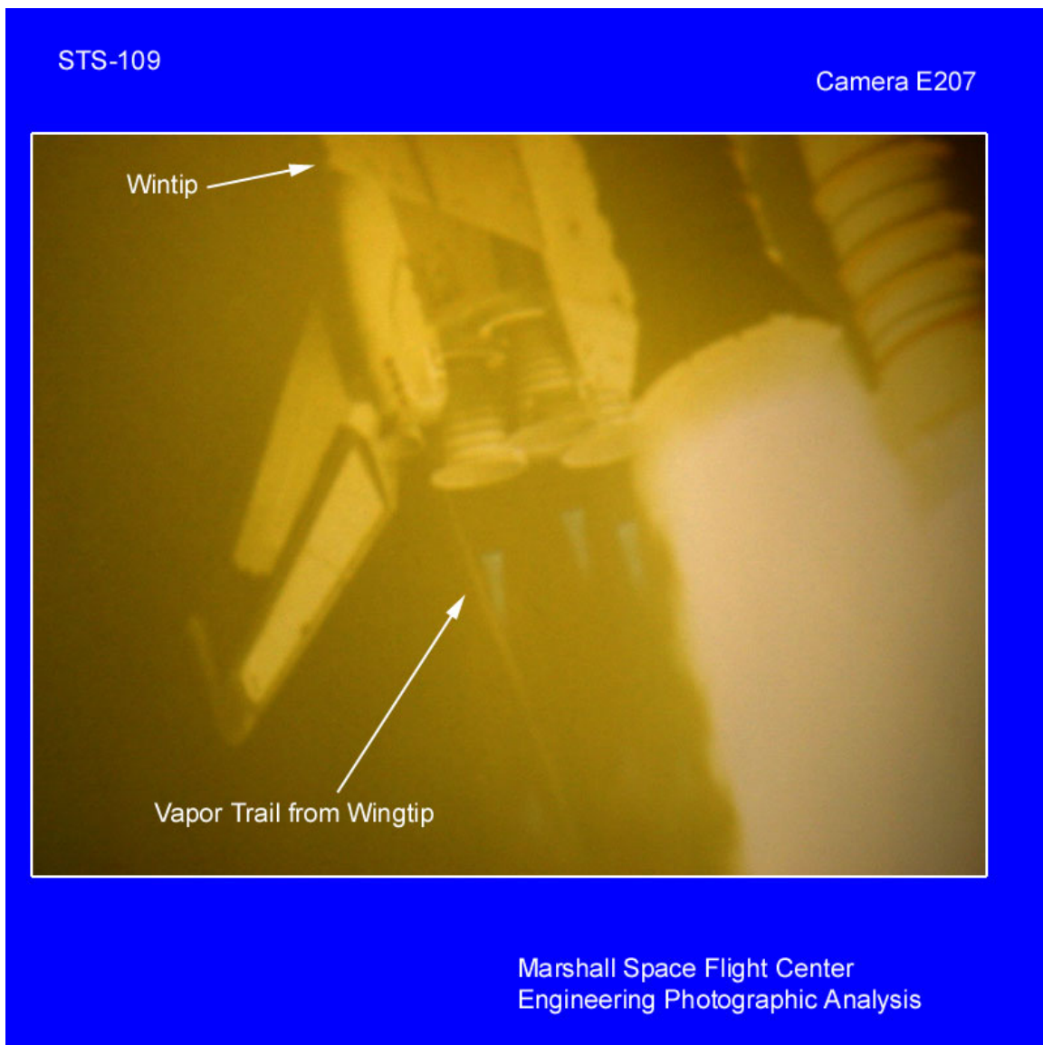
Figure 14. Film Camera E207: Vapors off Orbiter Wingtips
