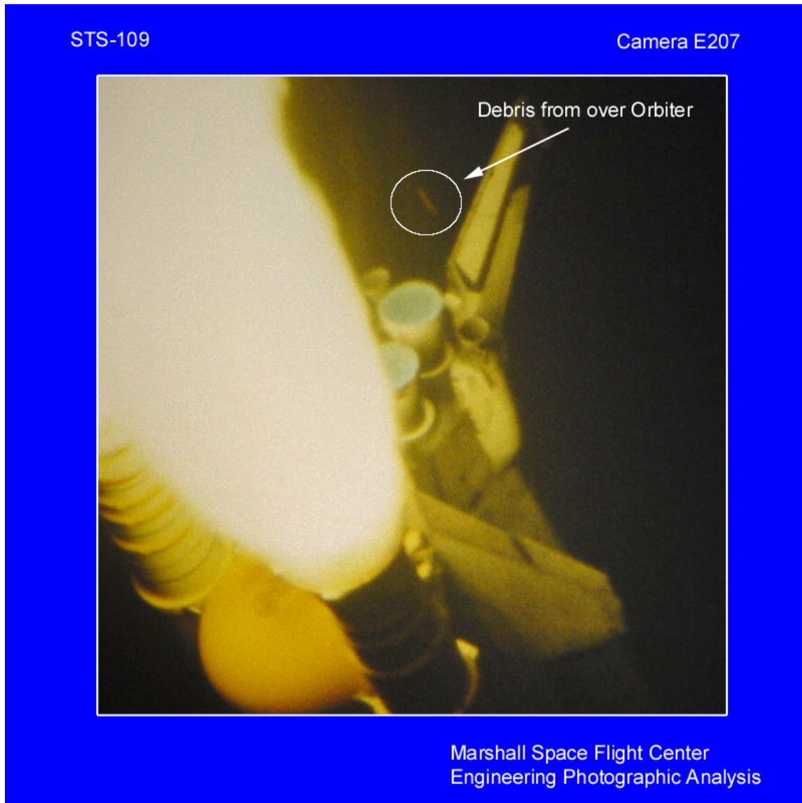
Figure 17. Film Camera E207: Debris Falling Aft
