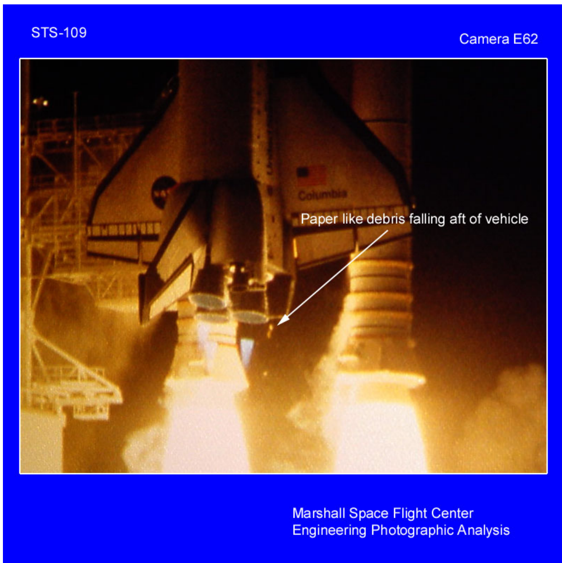
Figure 13. Film Camera E62: Debris Falling Aft
