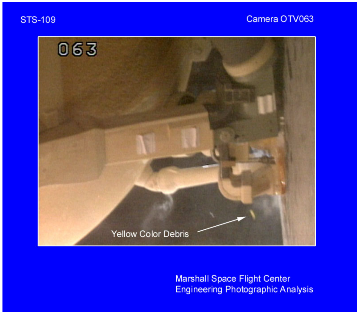
Figure 3. Video Camera OTV063: Yellow-Colored Debris
