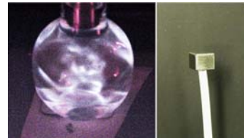
Figure 2: Radiation Detector Development: NASA GRC is attempting to verify claims of nuclear energy in sonoluminescence (left) using thin film coated scintillation detectors fabricated at NASA GRC (right).
