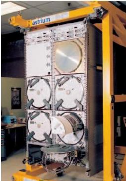
Figure 1. MELFI flight unit. One dewar door is open (bottom right) and a tray partially extracted.
