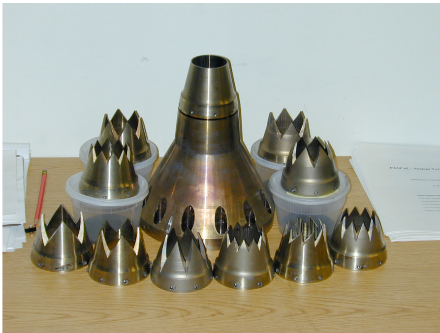
Figure 35.—The base nozzle with the SMC000 nozzle cone mounted (center) and a collection of chevron nozzle cones. The SMC nozzle system is far more economical, both in terms of building expense and model change time, than manufacturing a set of full nozzles.
