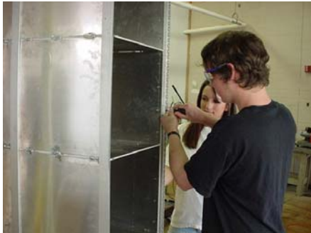
Two high school students working on an RSR that will be used for astronaut training at NASA JSC. RSRs are used within the multi-purpose logistics module (MPLM) to carry cargo to ISS aboard the space shuttle.
