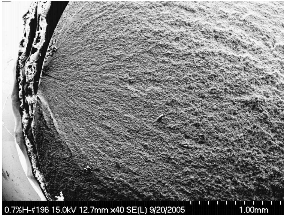
Figure 12.—Representative LCF fracture surface of hydrogen charged GRCop-84. (0.7% \Delta\epsilon_{\text{Total}} specimen tested in GH)
