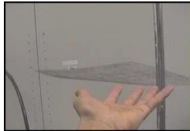
Carbon fiber \mu -truss fabric (1 gm/m 2 , 2 mm thick)
