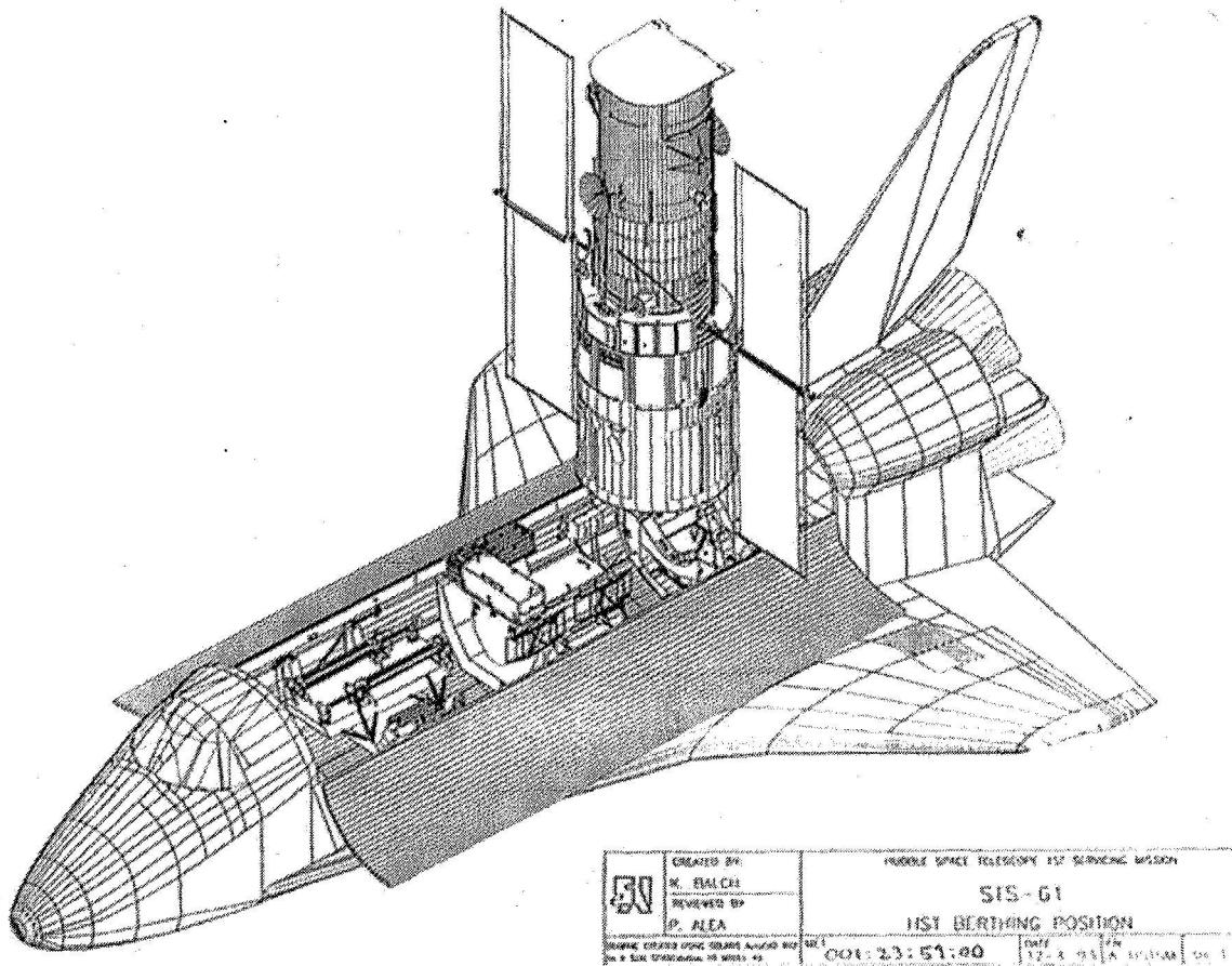
**Figure 2. Servicing Mission 1 Hardware Configuration.** The servicing carrier hardware is shown manifested in the Orbiter payload bay. The Solar Array Carrier is shown in the foreground, followed by the Orbital Replacement Unit Carrier. The HST is shown berthed on the Flight Support System.
