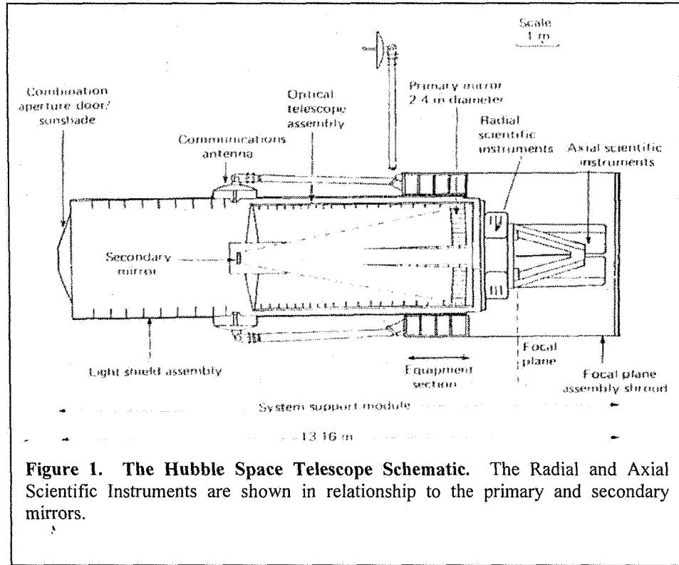
**Figure 1. The Hubble Space Telescope Schematic.** The Radial and Axial Scientific Instruments are shown in relationship to the primary and secondary mirrors.
