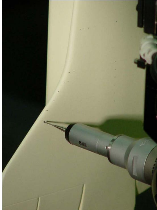
Figure 5: Placement of fiducial marks.
