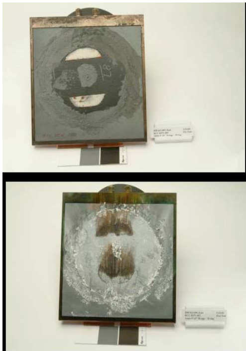
Figure 15. Arc jet tested plug repair.
