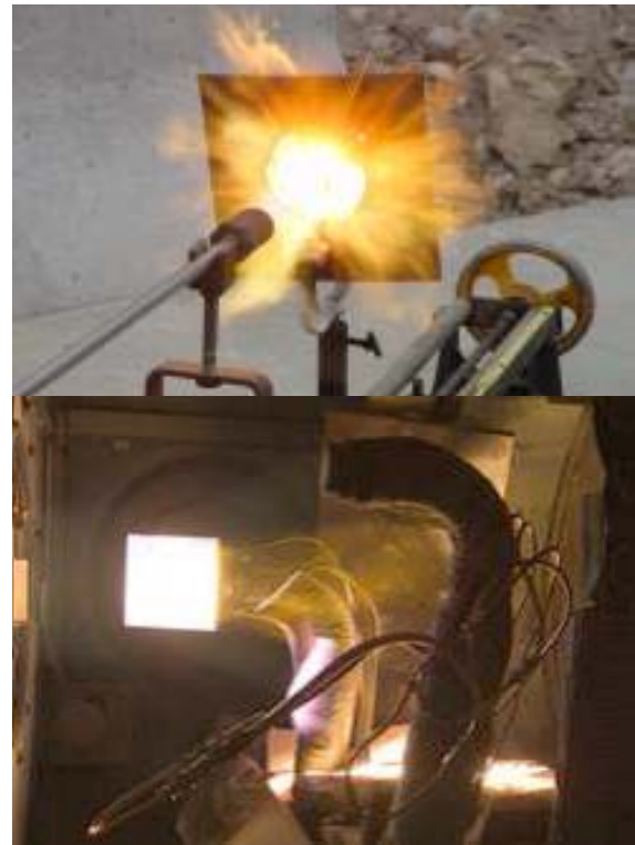
Figure 14. Typical torch and arc-jet tests.
