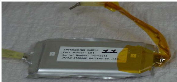
Figure 11. Laminate Pouch Cell after Overdischarge-into-Reversal Test.
