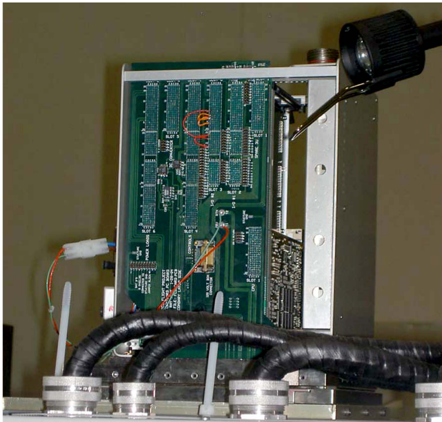
Figure 10.—View of PI box showing flexible circuit board.
