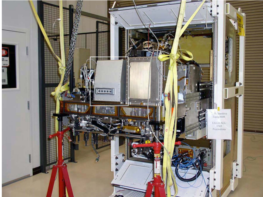
Figure 13.—PI box (highlighted) installed in cir engineering development unit.
