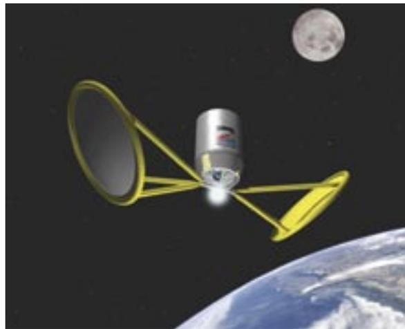
Harnessing the Sun's energy through solar thermal propulsion could propel vehicles through space by significantly reducing weight, complexity, and cost while boosting performance over current conventional upper stages. Pictured is an artist's conception of space flight using solar thermal propulsion.
