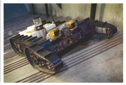
An autonomous stairclimbing behavior is used to take NASA's "Urbie" robot up multiple flights of stairs without any user control. This is accomplished with a combination of onboard sensors and vision algorithms to sense where the stairs are and which direction the robot should go to drive up the center of the stairs.
